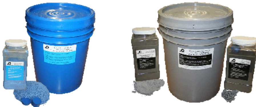
Figure 7-10 Glass-filled diallyl phthalate and epoxies have a glass filler to provide better edge retention during grinding and polishing.
