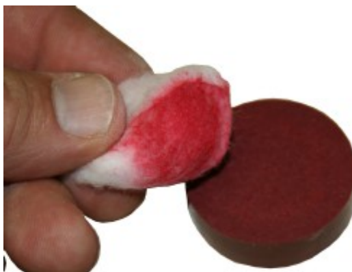
Figure 7-9 Insufficient curing of phenolic resin causes alcohol to dissolve the dye.
