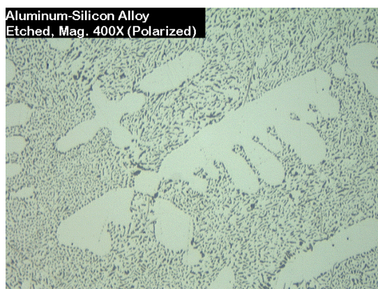
Aluminum - Silicon Alloy microstructure, Kallings etchant
