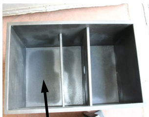
Three Chamber tank with counter-current flow
