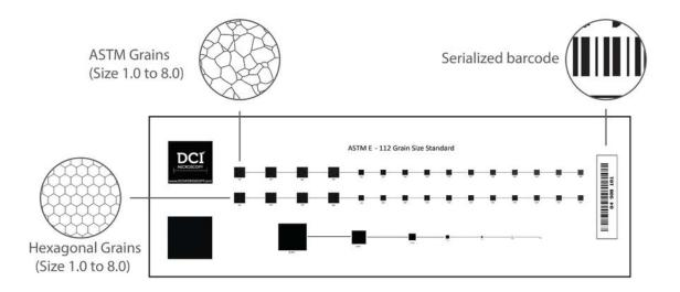
DCI Microscopy has developed a NIST-traceable calibration slide for the ASTM E-112 Grain Size measurement method. This slide will allow your quality control lab to validate the accuracy of your grain size measurements performed by image analysis on light microscopy-based systems. A certificate is supplied with the nominal value, and the measured value by both the planimetric and the Heyn method.
