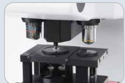
Unique Clemex self-level vise with built-in Test Block holder.
