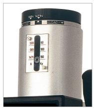
It is possible to carry out tests on any part even if small dimensioned. The visible indenter allows to reach extreme points for testing tool cutting edges as well. The bellow guard guarantees a constant and safe motion with no need of maintenance.
