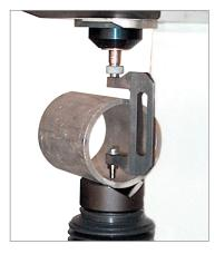
By applying C shape indenter Art. 604, difficult points as: insides of tubes and near to hollows can be reached.
